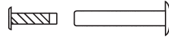
20-183 Rivet and Drive Screw Assy. Used when no rivet tool is available.
